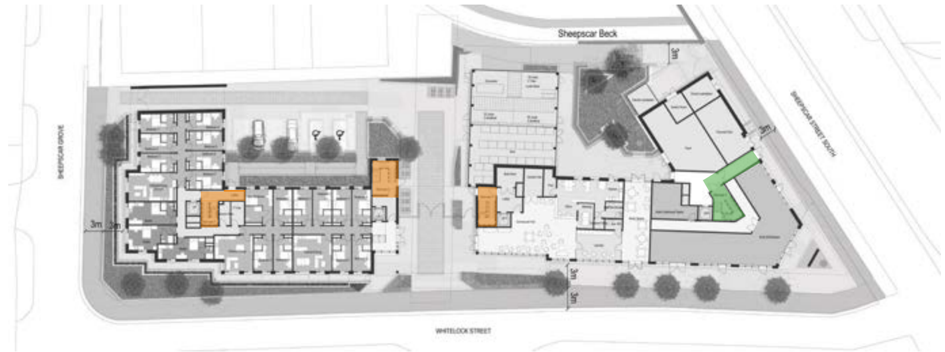
Stair Key Firefighting Stair Protected Stair
