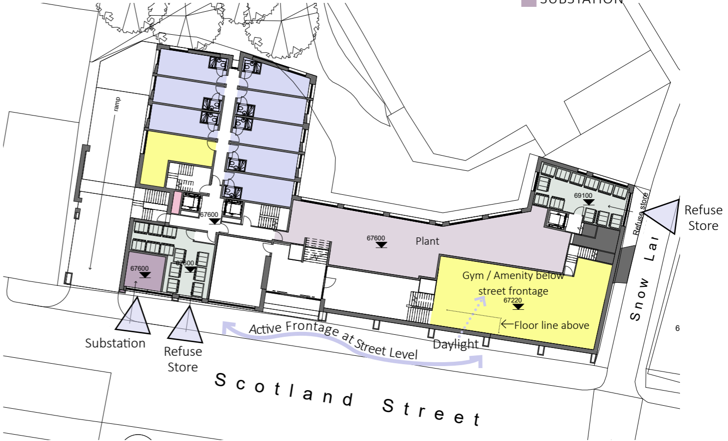
Level -1 Level access for substation on Scotland Street. Refuse store frontage minimised but maintain level access to Scotland Street to take bins out.
